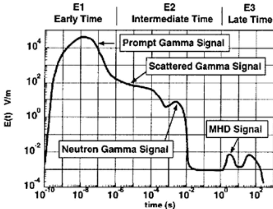
Figure 6: Composite EMP waveform from MIL-STD-464C.
