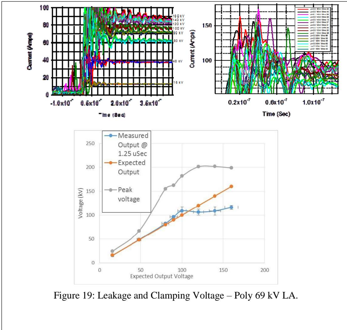
Figure 19: Leakage and Clamping Voltage – Poly 69 kV LA.
