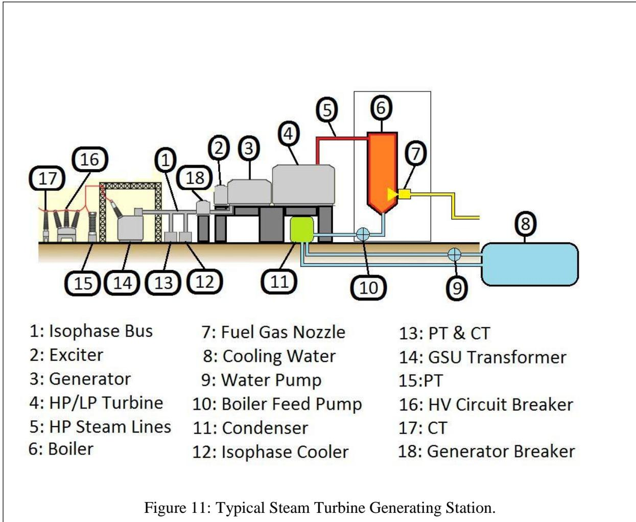
The Generating Station is connected to the high voltage switchyard via its generator step-up (GSU) transformer (see Figure 12-Figure 14). This transformer is typically a grounded-wye / delta configuration, with the delta on the generator side. While the GSU / substation will have nearby lightning arresters for protection, the grounded-wye configuration on the transmission grid network side of the transformer provides a path for the DC currents associated with E3.
