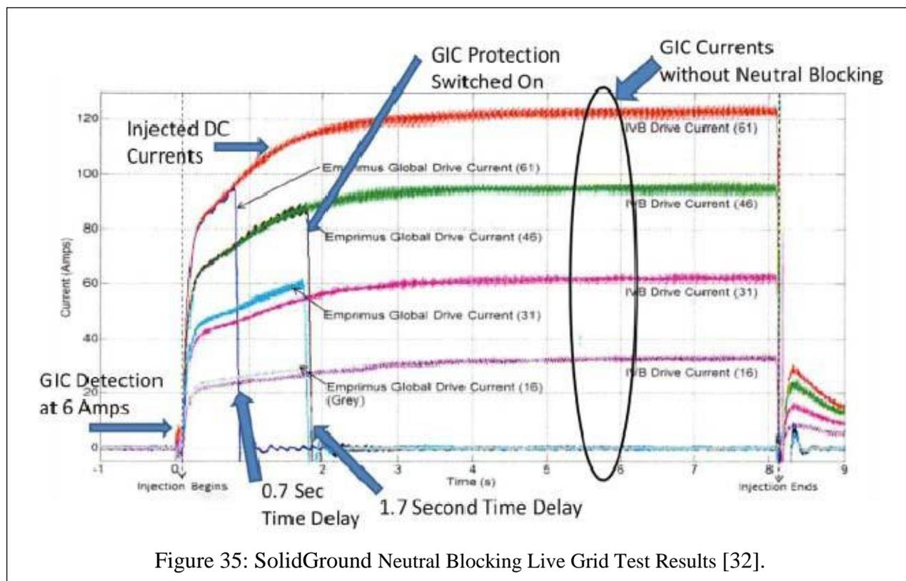
Figure 35: SolidGround Neutral Blocking Live Grid Test Results [32].
