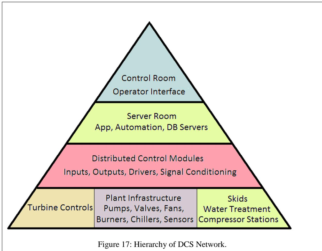
At the top levels of the DCS hierarchy, it is not uncommon for installations to use unshielded twisted pair (CAT5 or CAT6) cabling for connections between the operator interface console and the network hardware associated with the servers (though some will likely use shielded cable). Likewise, the servers may be interconnected via cabling that is unshielded, since the length of the runs will likely be short.
